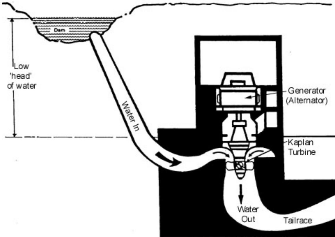
Figure 1c. Kaplan or propeller turbine installation.
