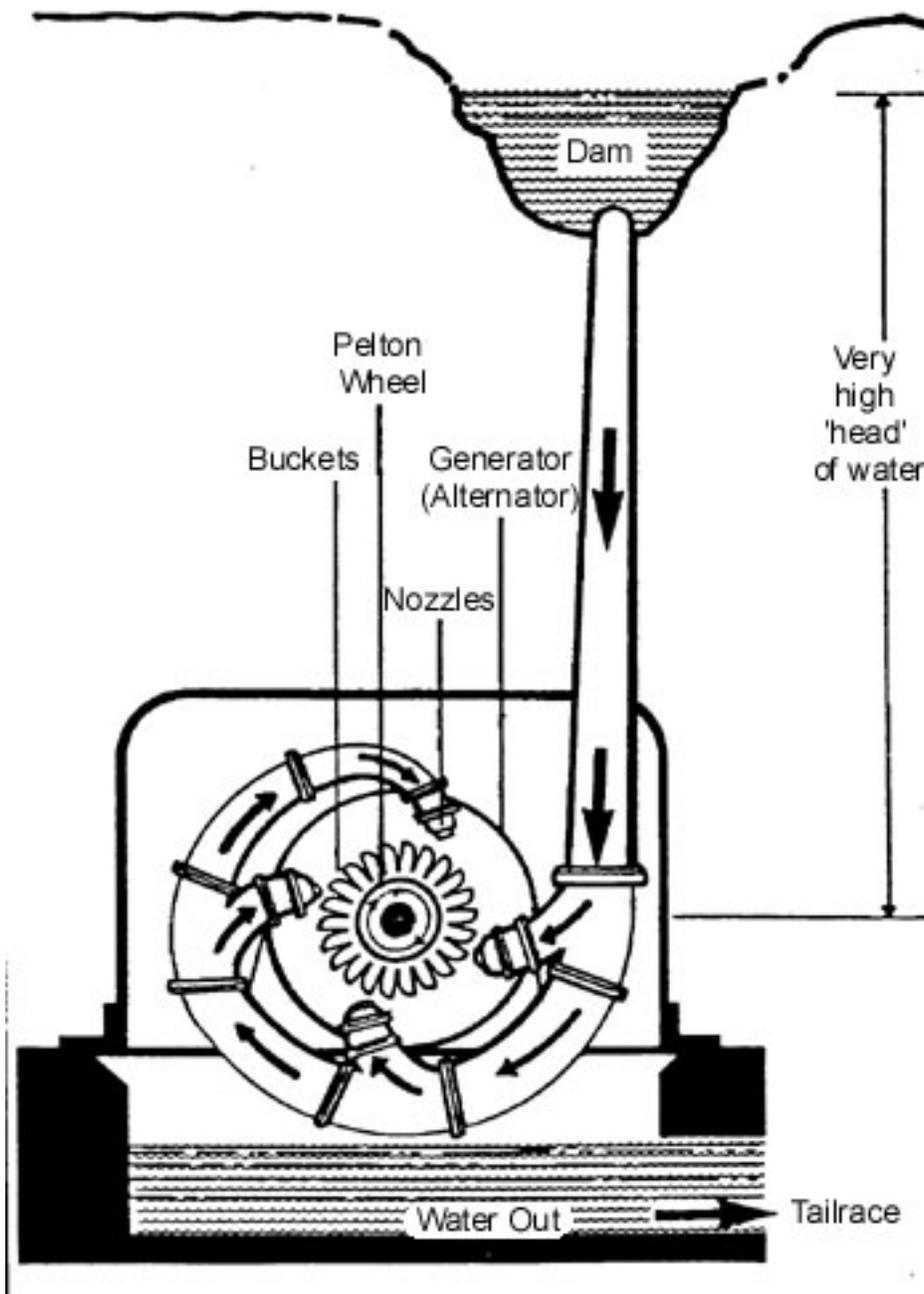
Figure 1a. Pelton wheel installation.
