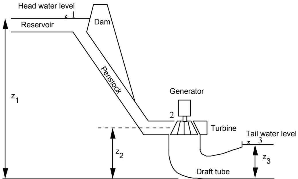
Figure 2. Schematic hydroelectric power plant.
