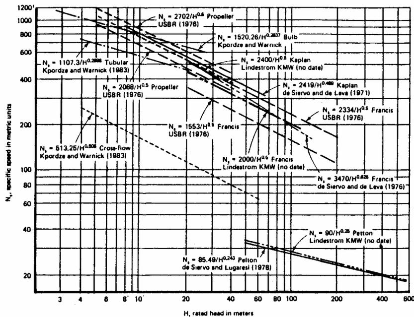
Figure 6. Specific speed correlations for various turbine types<sup>2</sup>.
