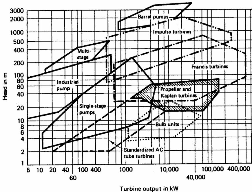
Figure 5. Turbine selection guide<sup>2</sup>.
