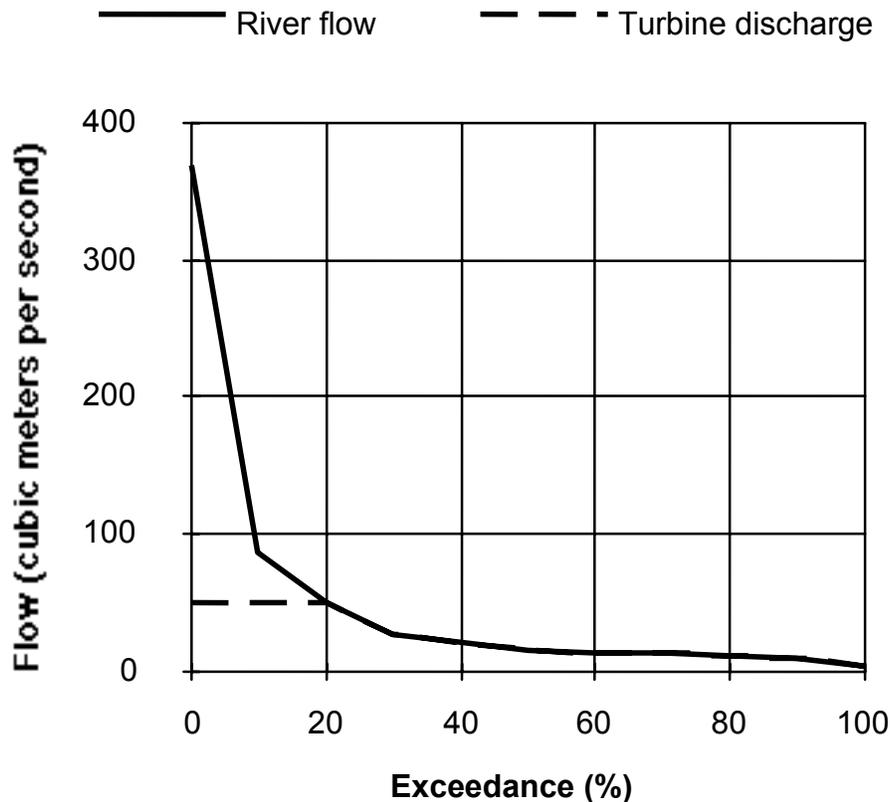
Figure 3. Stream flow duration and turbine discharge for the selection example.
