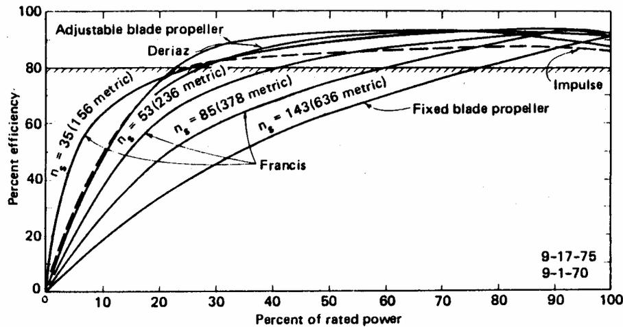
Figure 4. Hydraulic turbine efficiency<sup>2</sup>.
